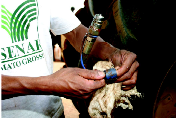
6.3 LIMPE A TAMPA DO CONECTOR MACHO
